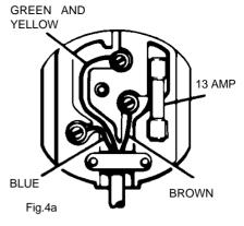
The wire which is coloured BROWN must be connected to the terminal which is marked with the letter 'L' or coloured RED.
